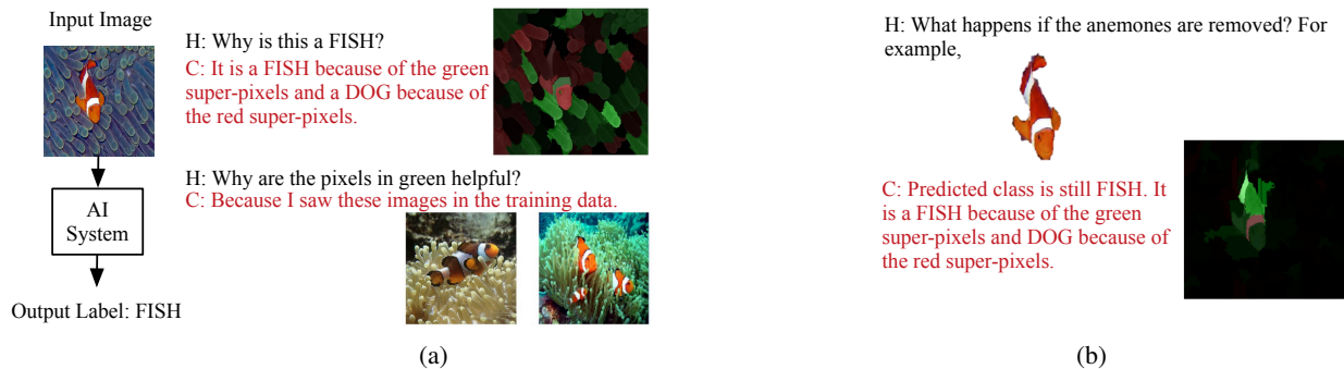
Figure 1: An example of an explanatory dialog for gaining insight into a dog/fish image classifier.
