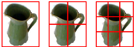
Fig. 5. Illustration of the spatial pyramid representation. A spatial EMK is the concatenation of EMK features computed over regions defined by a multi-level image decomposition. From left to right: 1 \times 1 , 2 \times 2 and 3 \times 3 decompositions.
